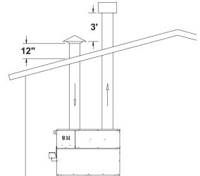
Figure 16 – Roof Top Combustion Air Inlet
